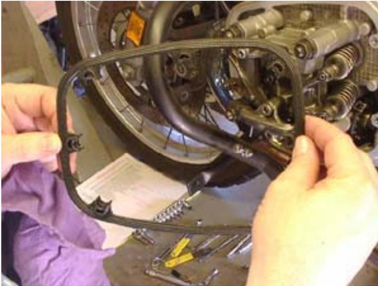
85. Put the rubber spark plug gasket back into/onto the cylinder head cover. You remembered to rotate this gasket so the plug indentations get virgin gasket, right? Ahhhh.
