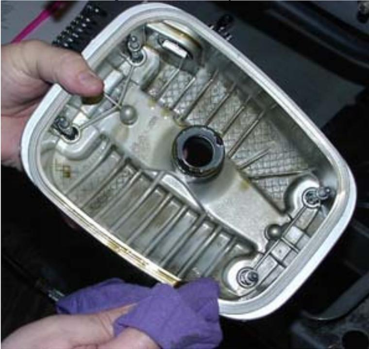
23. Now – some odd business. There's a rubber plug gasket that surrounds the spark plug. It's typically stuck to the inside of the cylinder head cover, but it might still be buried in the head in the spark plug tunnel.
