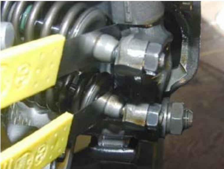
44. Make sure all four feelers are in place at the same time. In this picture, the front of the bike is on the left, meaning the exhaust valve assembly is on the left and the intake valve assembly is on the right.
