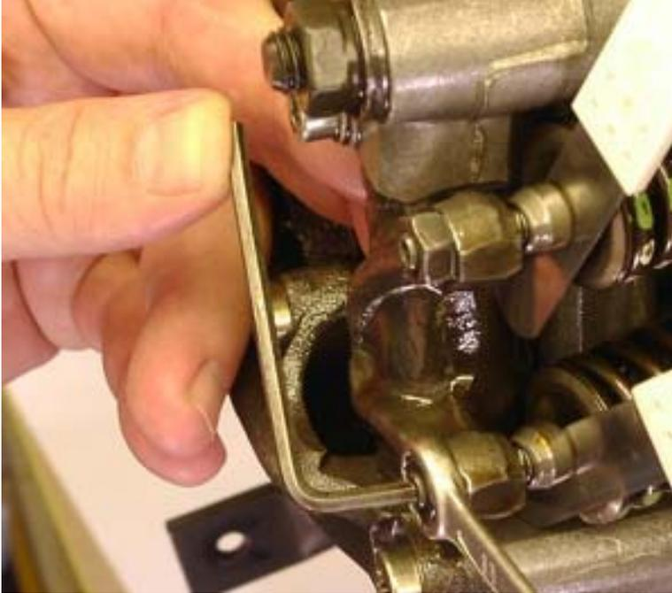
58. Loosen the lock nut with the box wrench.
