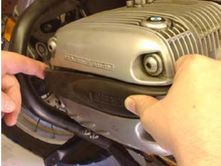
Once the rubber insert is seated into the back of the cylinder head cover, you can just apply a little pressure laterally along the side of the cylinder head and the cover will just snap into place. Und voila, amigos! Ich neyt parlez pas Spanglais!
