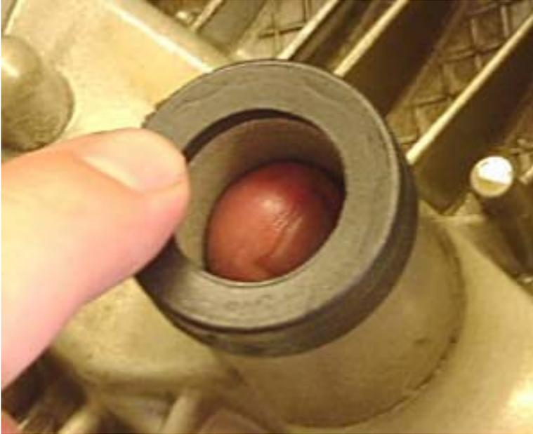
86. Pop the cylinder head cover back on the bike. Remember there's oil in it. Get all your surfaces together with hand pressure, then start tightening bolts. Don't dawdle. **Faster**, damnit!
