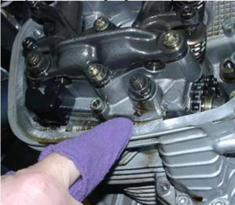
22. Clean the matching surfaces on the cylinder head cover.
