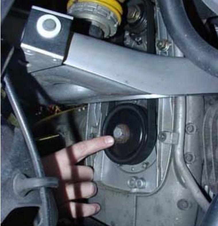
9. You'll find the engine timing hole on the 'Throttle grip' side of the engine. It's that little round slightly concave rubber plug behind the cylinder head, right up above the throttle body, just below the telelever hinge. Oh, for chrissakes, it's right HERE...
